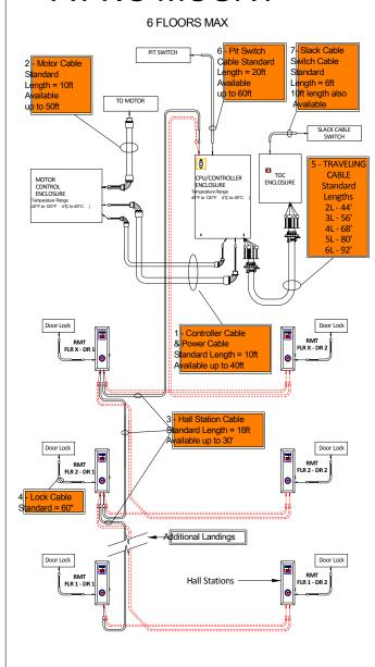
Cable lengths shown are standard based on number of landings ordered. Inclinator offers additional cable length options to meet non-standard installations. Please see order form for additional information on longer cable lengths
