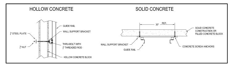
NOTE: All mounting points should meet or exceed the minimum pull out force for all rail reactions.
